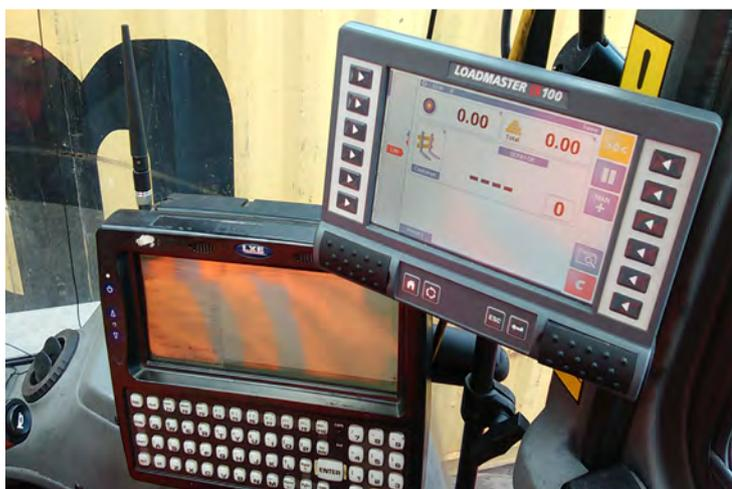
**A dynamic on-board weighing system specifically designed for forklifts that meets SOLAS Method 2 requirements**
