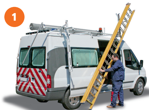
1 - Put the ladder on the front support;
