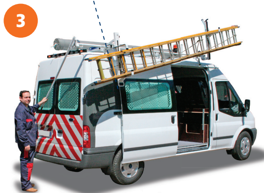
3 - High roof vehicles: lift the slide upwards until it is fixed;
